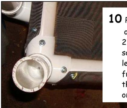
**10** Place 2 screws on the bottom of 2 opposite corners so they hold the legs & stop them from turning under the weight of dog on bed.
